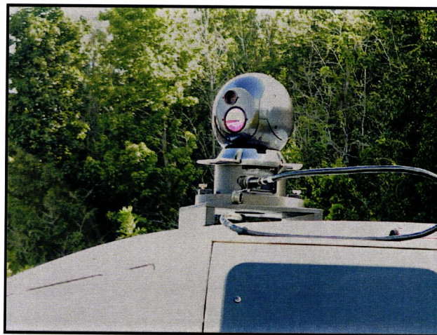
Figure 9 Ball Turret Camera Mounted on Roof
